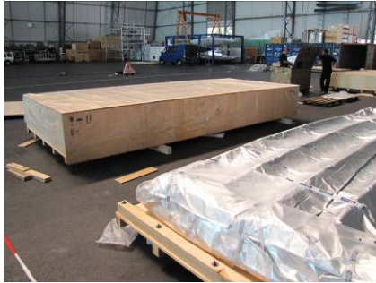
Special, tailor-made: Transport box for Zeppelin longerons
